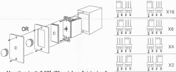
Mounting depth: 2.87" (73mm) from finished wall.
